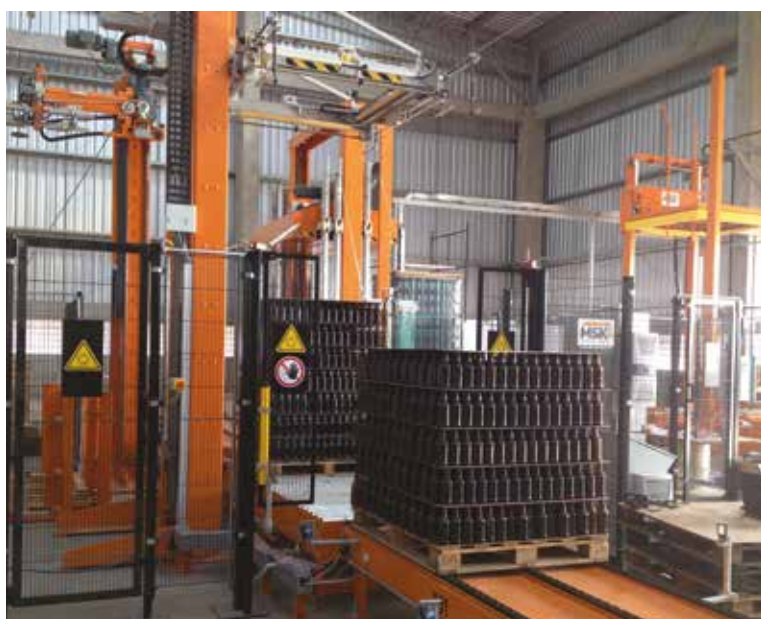
For the third production shop at Vidroporto, MSK delivered the complete cold end from the Lehr exit to pallet packaging.
